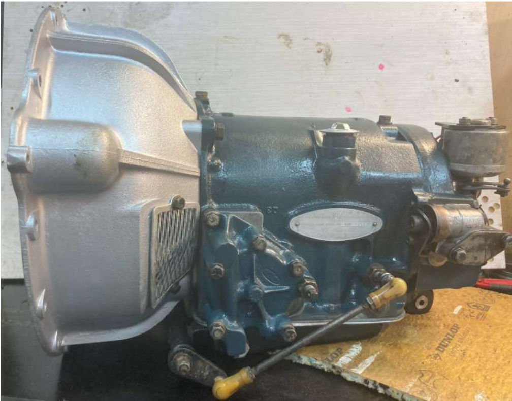
Completed DG Transmission
