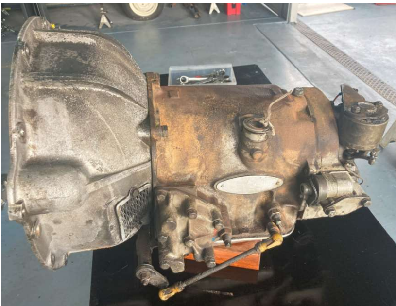
Faulty DG Transmission Before stripping.
