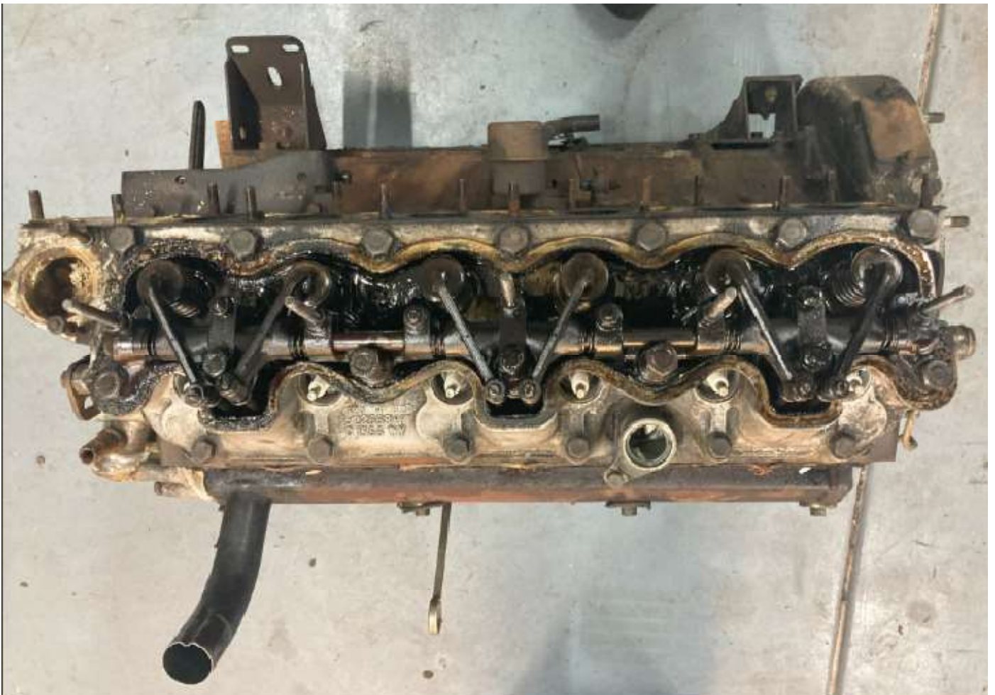
3 Litre P5 engine at the start of dismantling.
